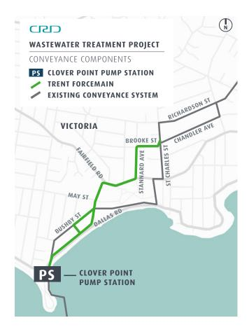
The pipe will be installed along the Dallas Road Waterfront Trail from the Clover Point Pump Station to Eberts Street. The waterfront trail will be closed during construction but access to the beach will remain open. Following construction, the trail will be restored to its original condition.
