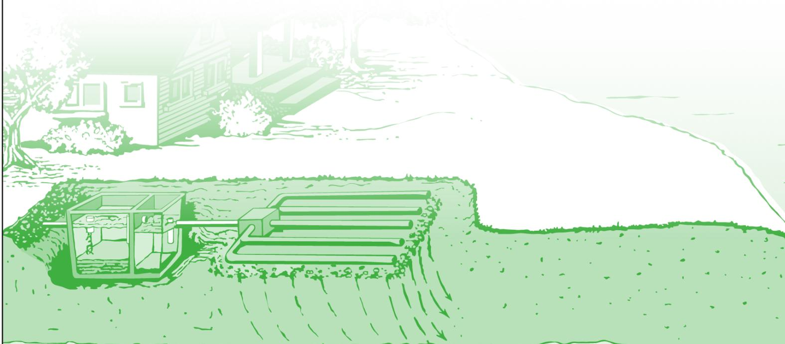
**5. Can I build a carport or camper pad over the drainfield? How about a tennis court or a hot tub?** No, for two reasons. First, you should avoid driving over the drainfield. The pressure of vehicles and heavy equipment compact the soil and can damage pipes. Second, impermeable materials such as concrete and asphalt reduce evaporation and the supply of oxygen to the soil. Oxygen is critical to the proper breakdown of sewage by soil microorganisms.
