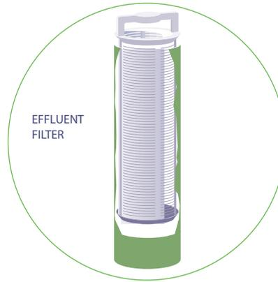
**10. How does an effluent filter protect my drainfield?** An effluent filter fits securely in your outlet T and is highly effective at keeping solids out of the drainfield. It forces the wastewater to pass through small holes before entering the
