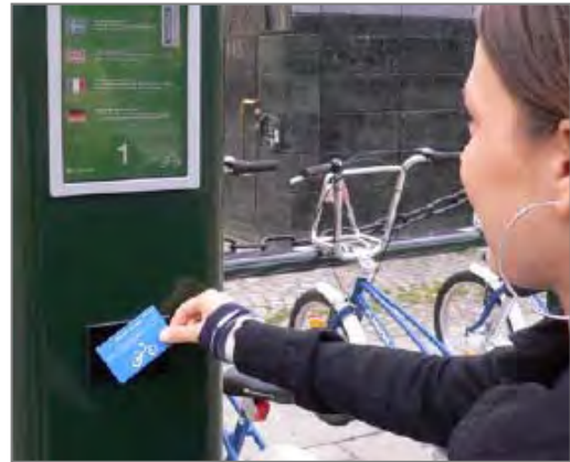
Figure 18. Check-in/check-out procedures at a card-access kiosk. Instructions are available in several languages.
