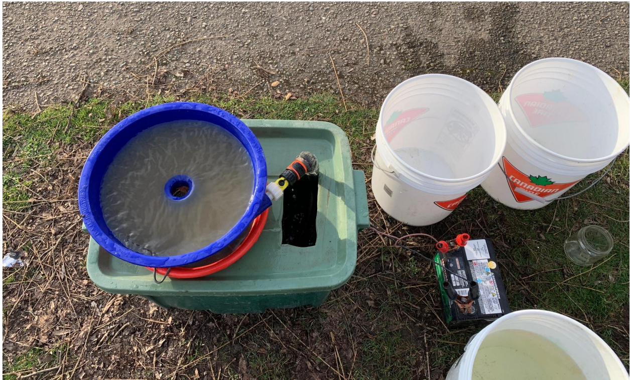
Figure 5. The vortex blue bowl system set up to separate forage fish eggs from sand. The process begins with the sample being swirled in the blue bowl vortex. The red 0.5 mm sieve collected all eggs and any other lighter material which float to the top of the vortex. The contents of this sieve were then analyzed under a microscope at home (Photo by Molly Duncan taken on March 8, 2021).
