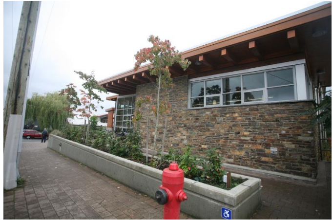
Figure 2 Planter watered by roof water captured in underground detention tank, Salt Spring Island Library
