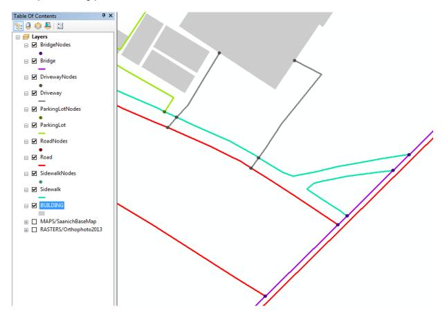
Example showing planimetric feature start and end nodes:
