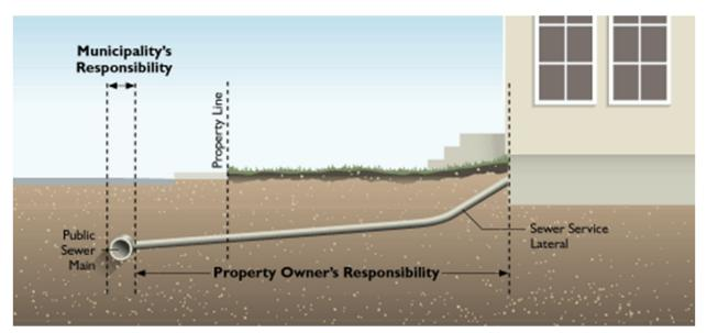
Municipalities and regional districts generally have mature programs for inspecting, maintaining, and replacing their sewer pipes. In contrast, property owners rarely inspect or repair their laterals unless there has been a pipe failure or blockage.
