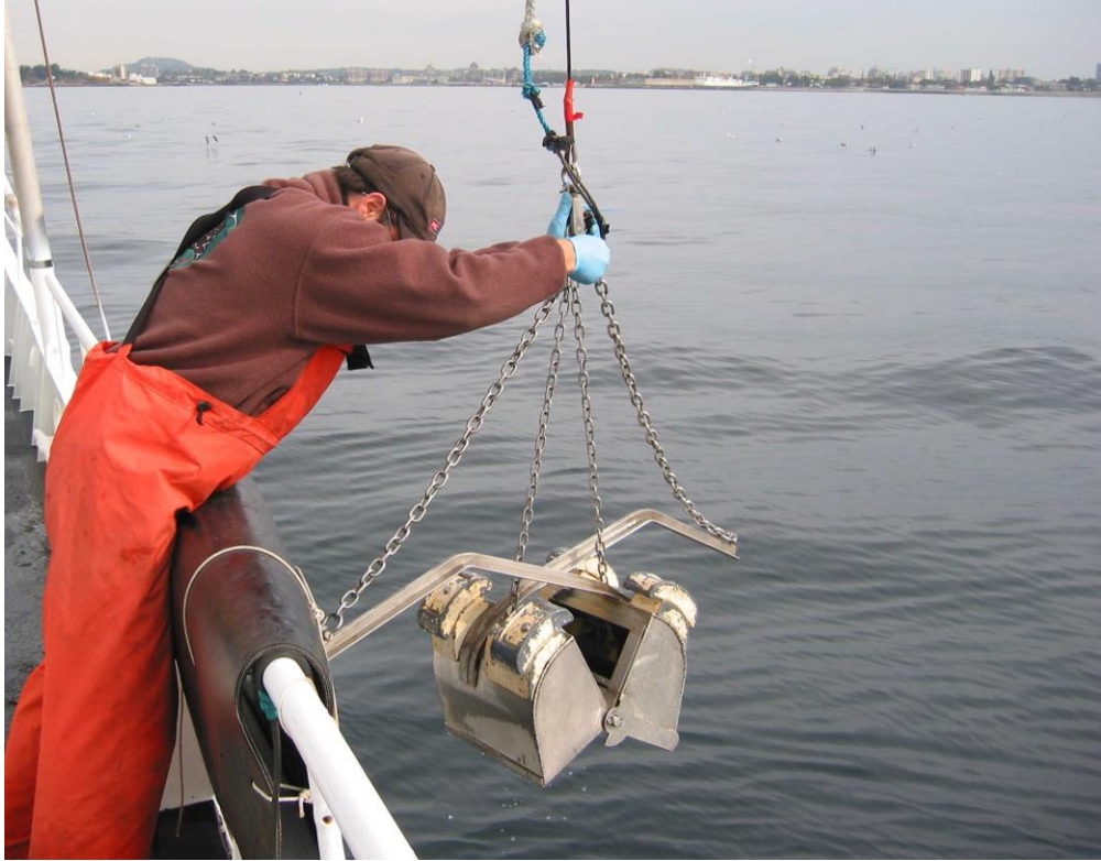
Picture 5.1 Seafloor Sampling Van Veen Grab
