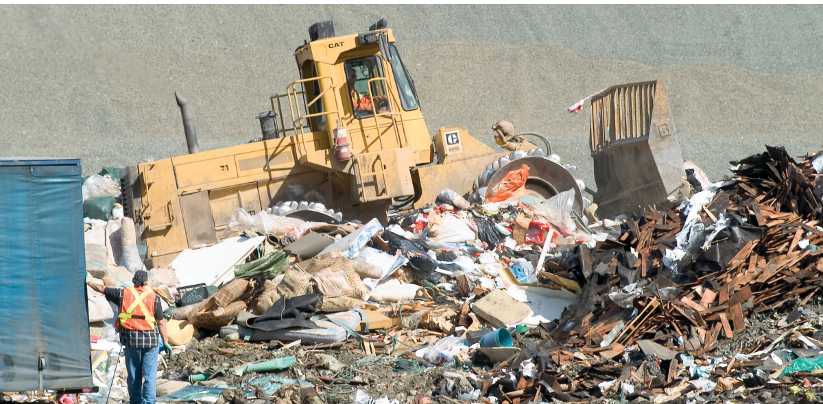
Compactor at Hartland's active face.
