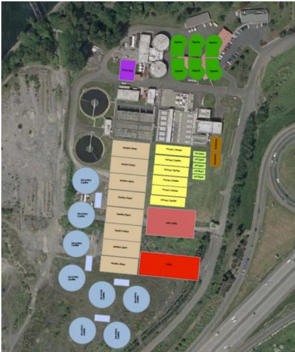
Figure 16: Conventional Activated Sludge Build-out Site Requirements
