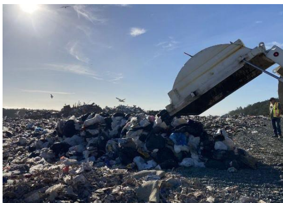
Figure 2-1: SF Load Tipped on Designated Tip Face Area
