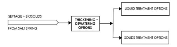
Figure P. Process Component Options Diagram
