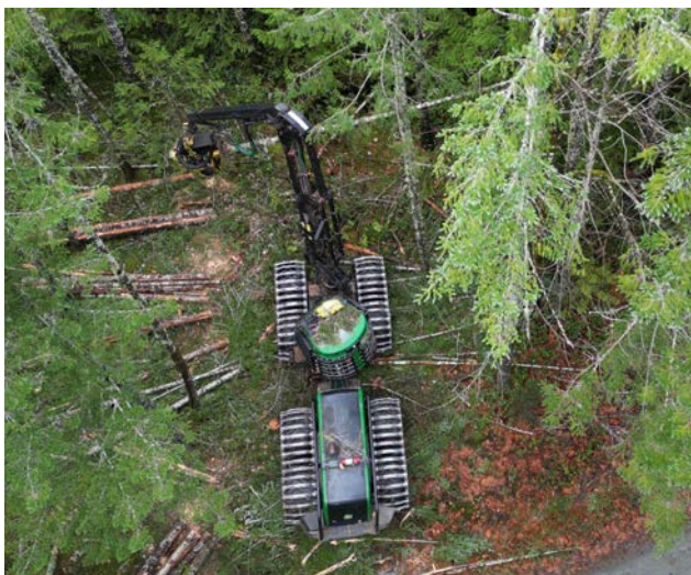
View of the narrow harvester with low ground pressure tracks and long boom for thinning.
