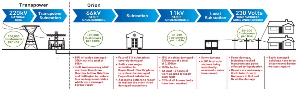
Figure 6 - Christchurch, New Zealand 2011 Earthquake Electrical Grid Damage [29]
