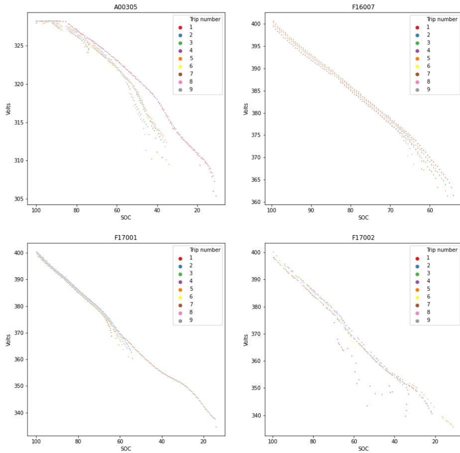
Figure 5: EV example trips showing the broad relationship of SOC vs the main battery's voltage
