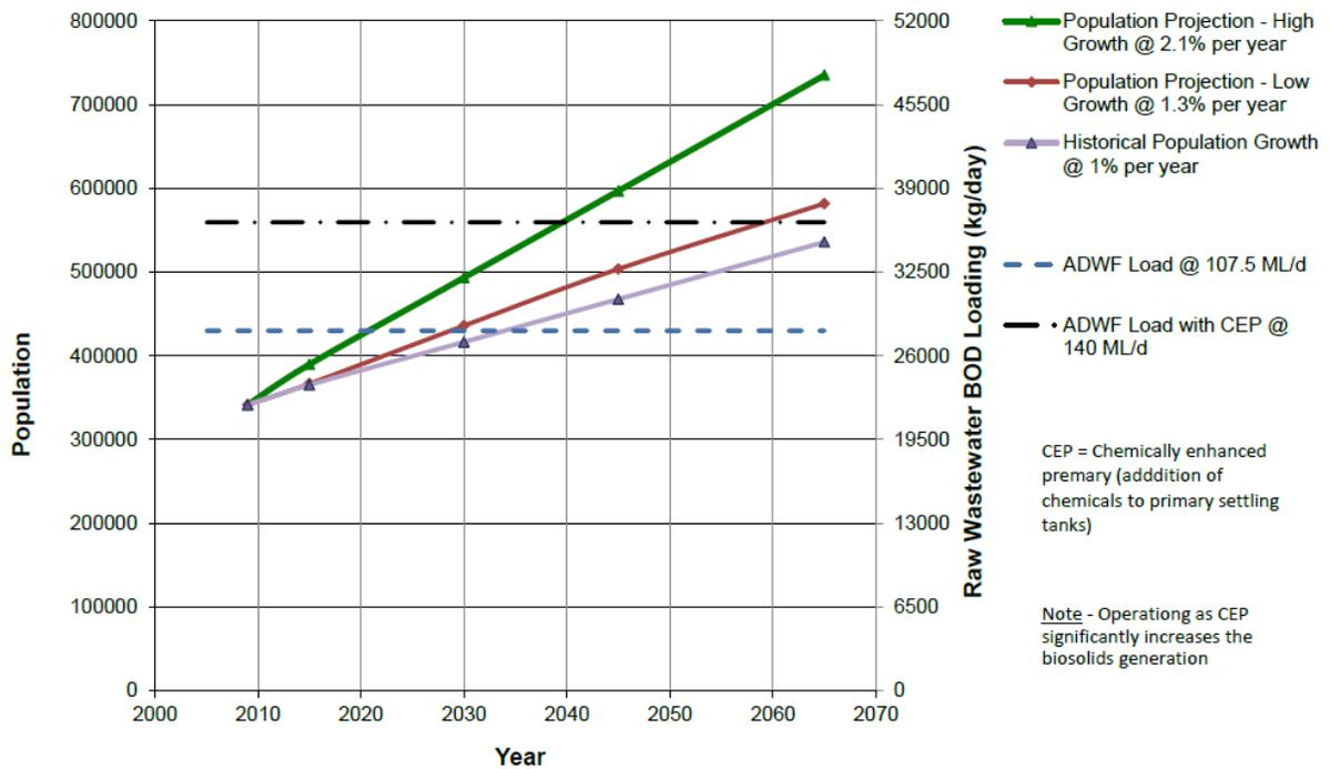
The average dry weather load for a 107.5 ML/day plant of 27,950 kg/day is represented by the blue dashed horizontal line on the graph.
