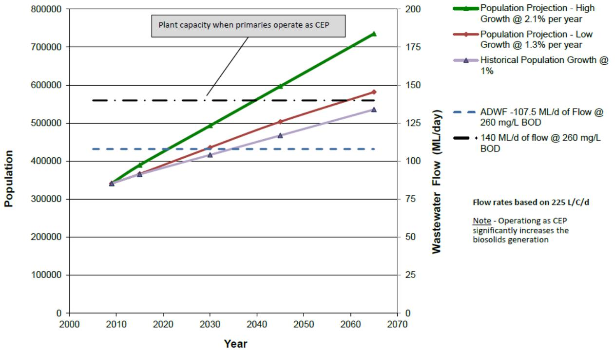
Operating the primary clarifiers as CEP facilities significantly increases the ability to handle increased loadings equivalent to the loading from a 140 ML/day plant, which stretches the life line of the plant to 2040 for the high growth scenario and 2060 and 2065 for the most probable growth and low growth rate respectively. If water reductions were incorporated, these life lines would be stretched even further into the future. Essentially Figure 2 is echoing the same conclusions as Figure 1.
