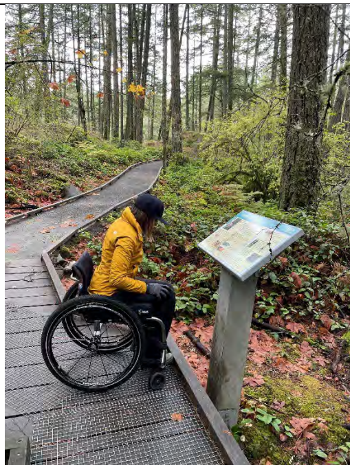
Positioning of Interpretive Signage Can Limit Ability of Some Visitors to Engage with the Sign
