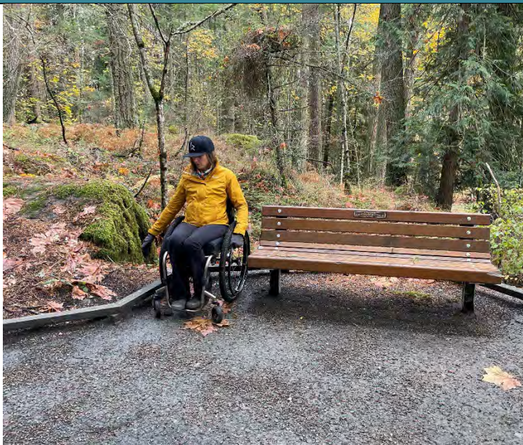
Benches Installation Should Include Space on Either End to Accommodate Mobility Devices
