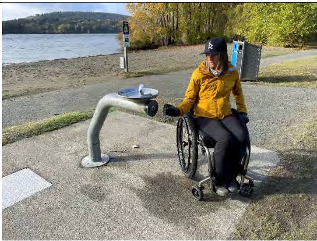
Inaccessible Open / Close Mechanism on Waste Receptacle – Some Visitors Do Not Have the Core Strength to Open the Lid
