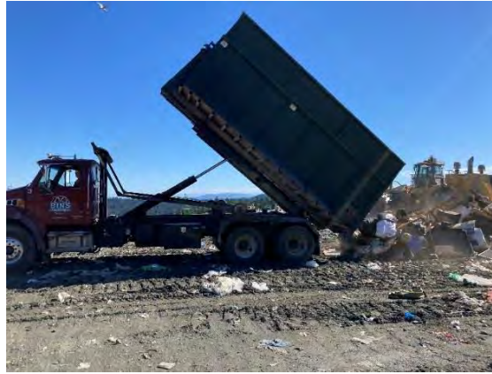
Figure 2-4: Public Drop Off Load Tipped on Designated Tip Face Area
