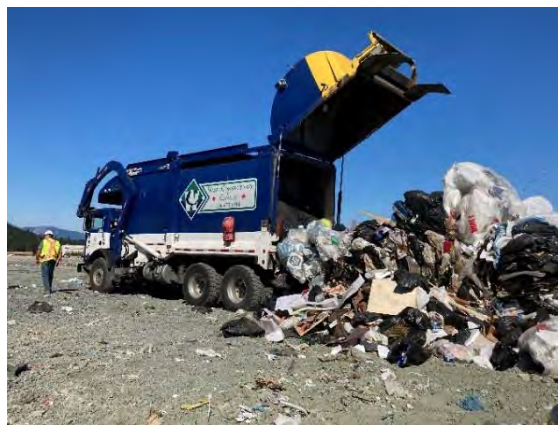
Figure 2-3: ICI Load Tipped on Designated Tip Face Area
