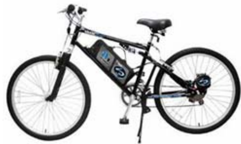
Figure 1. A motor-assisted cycle requires the user to pedal.
