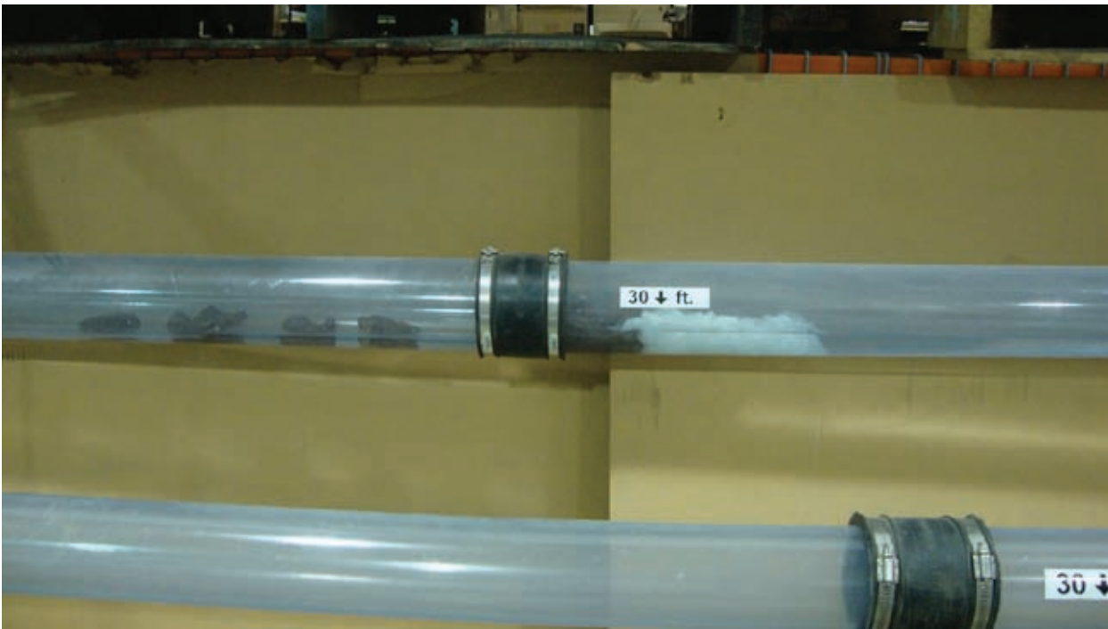
PHOTO 7-F ORDERLY FLOW OF SOLIDS IN TEST RUN #1 @ 1.6 GALLON (6.0 L) VOLUME, 1% SLOPE
