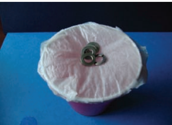
PHOTOS 7-G - TOILET PAPER WET TENSILE STRENGTH TEST
