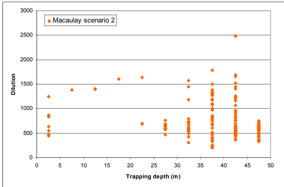
Figure 5.13 Scatter diagram of dilution versus trapping depth for the Macaulay outfall for the scenario 2 simulation.
