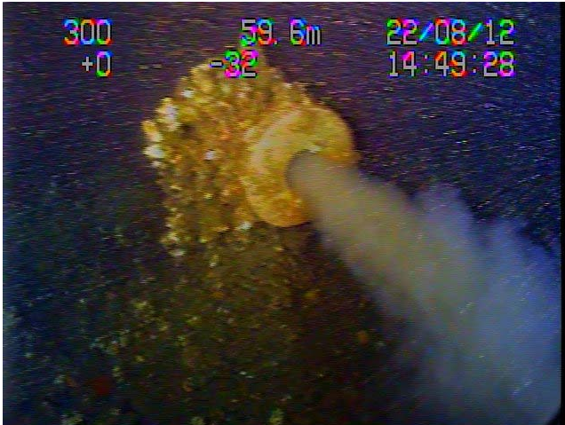
Photo A Effluent Jet Discharged from Clover Point Outfall Diffuser Port
