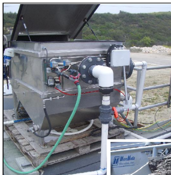
CleanScreen - see shipping skid as a scale for footprint.
