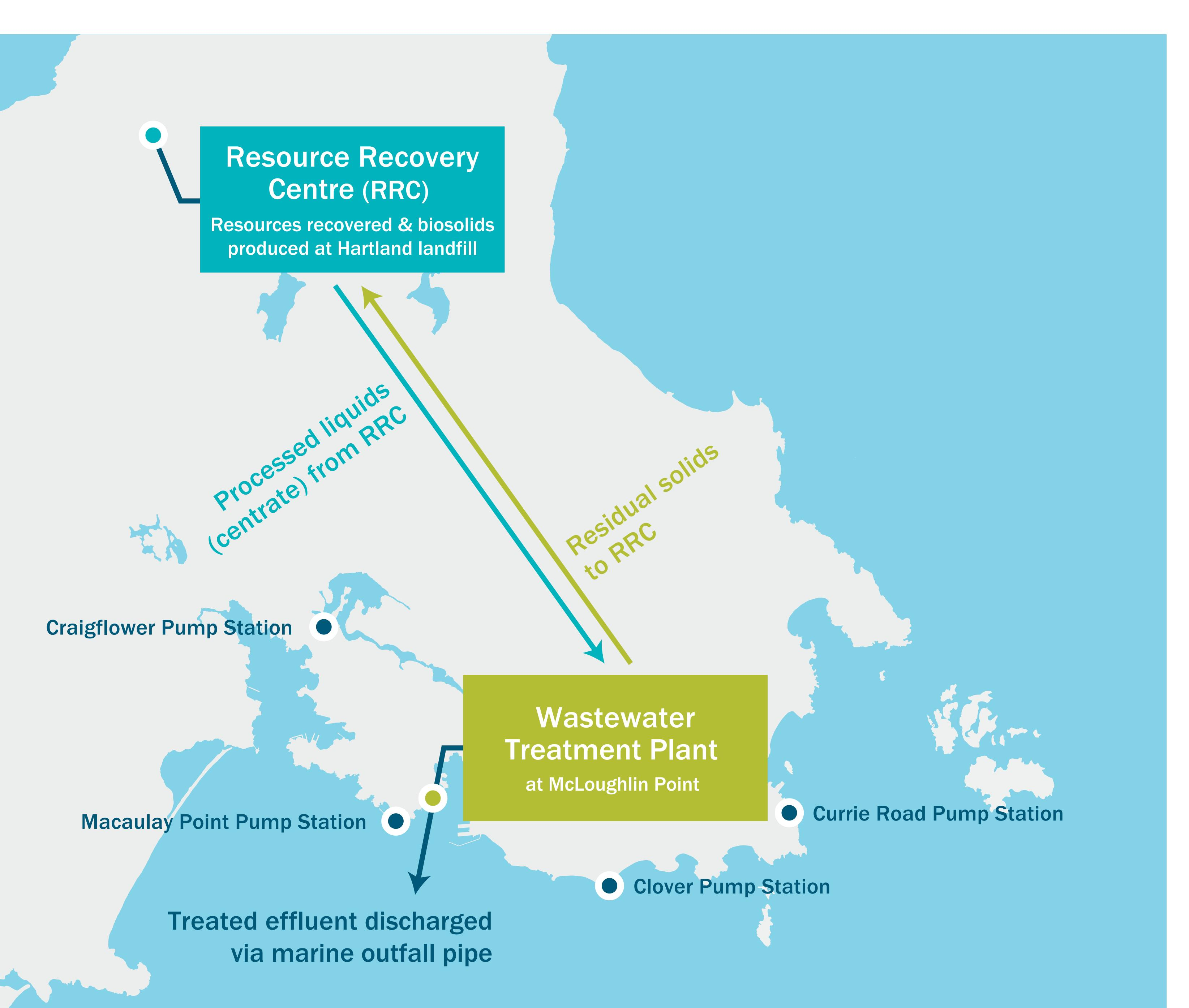
An underground pipe will transport residual solids from the Wastewater Treatment Plant at McLoughlin Point to the RRC. The residual solids are made up mostly of water (only 2% solids). Water extracted from the residual solids processed at the RRC will be piped back to the Treatment plant at McLoughlin Point. No wastewater will be released at Hartland landfill.
