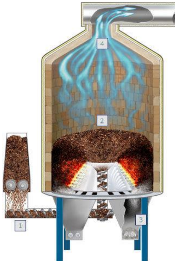
Figure 3.19 – Nexterra Gasification Process
