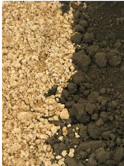
Figure 3.7 – Lime-stabilized Biosolids (left) Compared to Biosolids without Lime (right) (source: OMRR, 2008)
