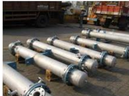
Figure 10.2 Diagram and Photos of Shell and Tube Heat Exchangers
