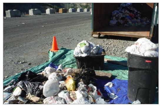
Photo 5: Collection of a Sample from the Waste Dumped by the Loader Operator
