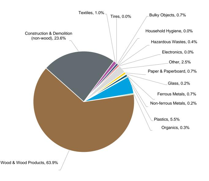
Figure 5: Primary Category Composition – Construction, Renovation and Demolition (N=20)
