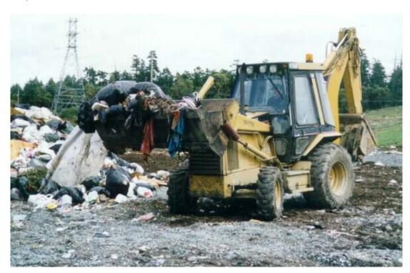
Photo 2-1. Backhoe with Three Way Front Bucket Loading Sample
