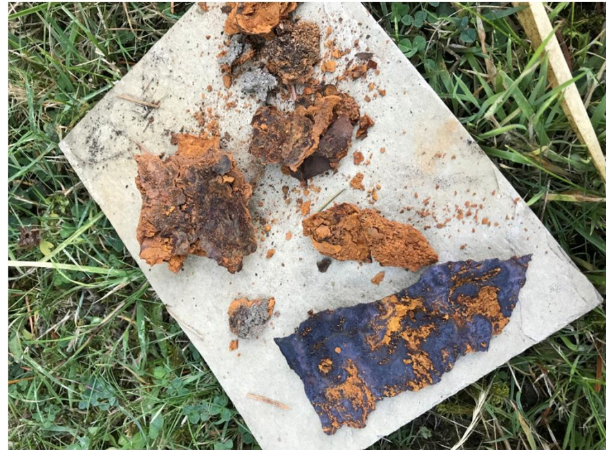
Photograph #6: 50 mm dia. Irrigation feed View of samples collected from pipe spool
