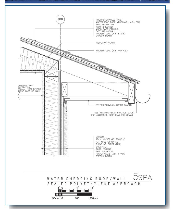
Detail 5 SPA: Water Shedding Roof/Wall-Sealed Polyethylene Approach
