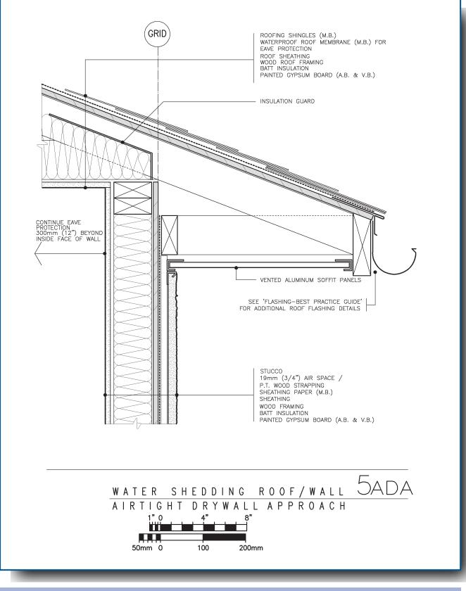
Detail 5 ADA: Water Shedding Roof/Wall-Airtight Drywall Approach
