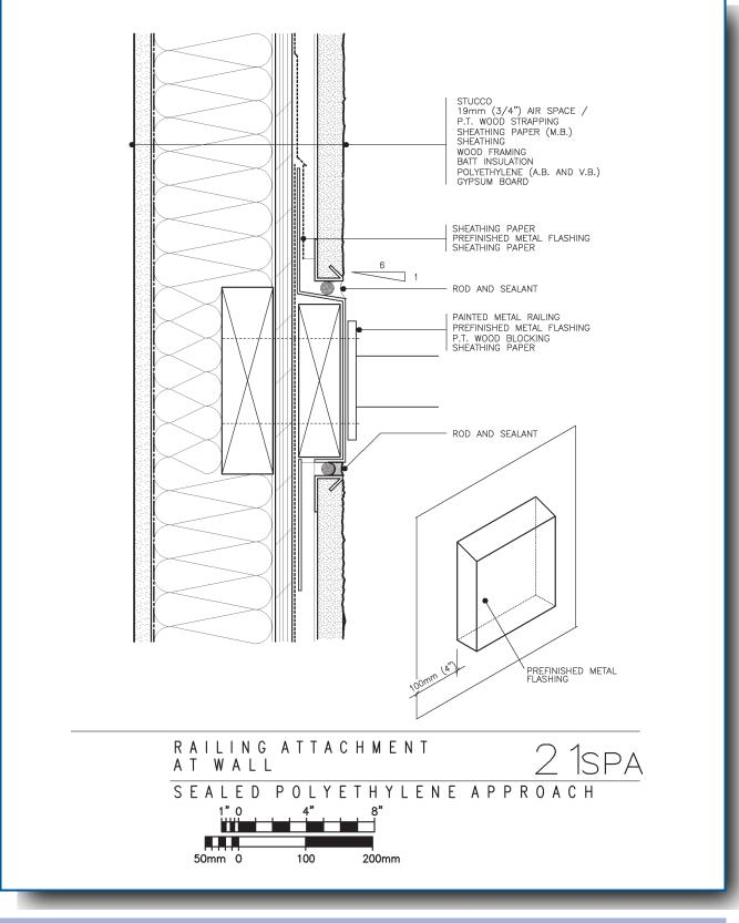
Detail 21 SPA: Railing Attachment at Wall-Sealed Polyethylene Approach
