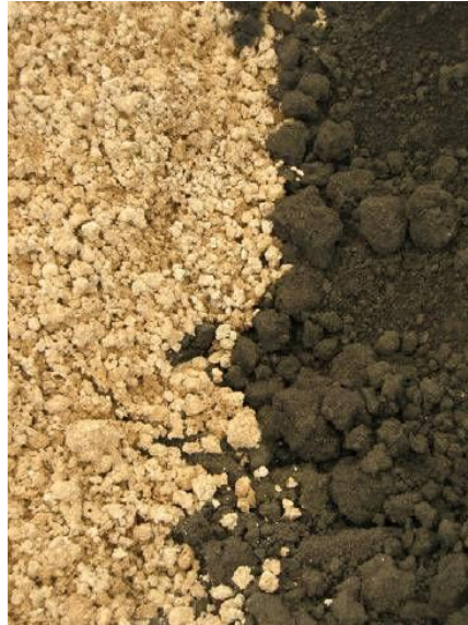
Figure 3.7 – Lime-stabilized Biosolids (left) Compared to Biosolids without Lime (right)
