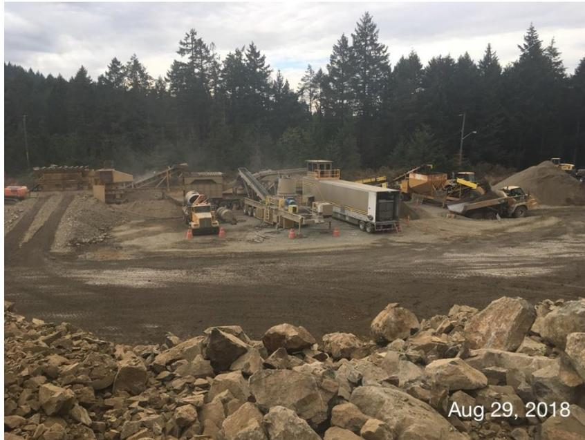
*Figure 9 – Rock crushing plant in operation.*
