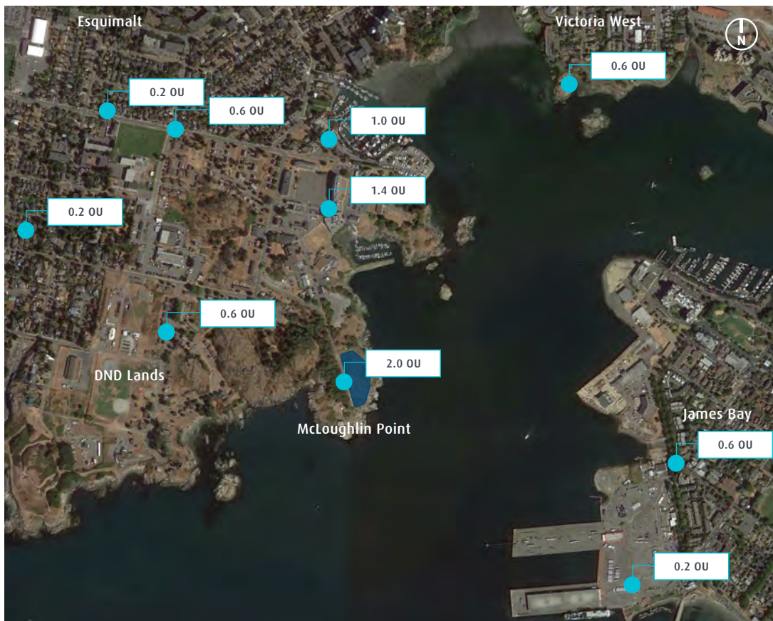
Odour from McLoughlin Point Wastewater Treatment Plant. Odour model based on the worst-case wind conditions over the last five years, based on regional meteorological data.
