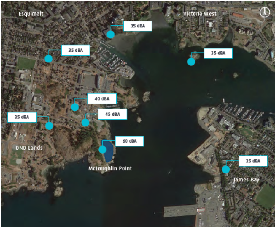
Predicted noise from McLoughlin Point Wastewater Treatment Plant. The noise model was generated with the state-of-the-art acoustical modelling software CadnaA which performs sound propagation calculations according to the widely used international standard ISO 9613-2:1996.
