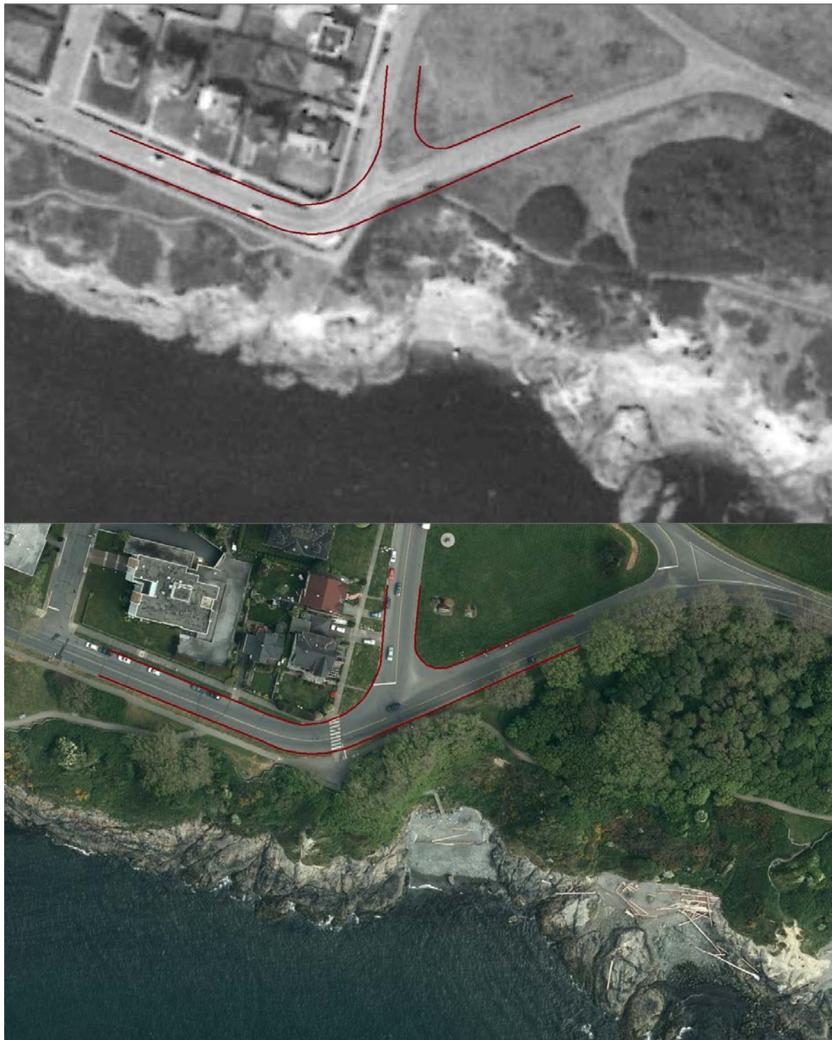
Figure 6 Comparison of 1956 air photo and 2015 orthophoto at Douglas Street and Dallas Road intersection. Red lines indicate the curb-to-curb extent of Dallas Road for reference.
