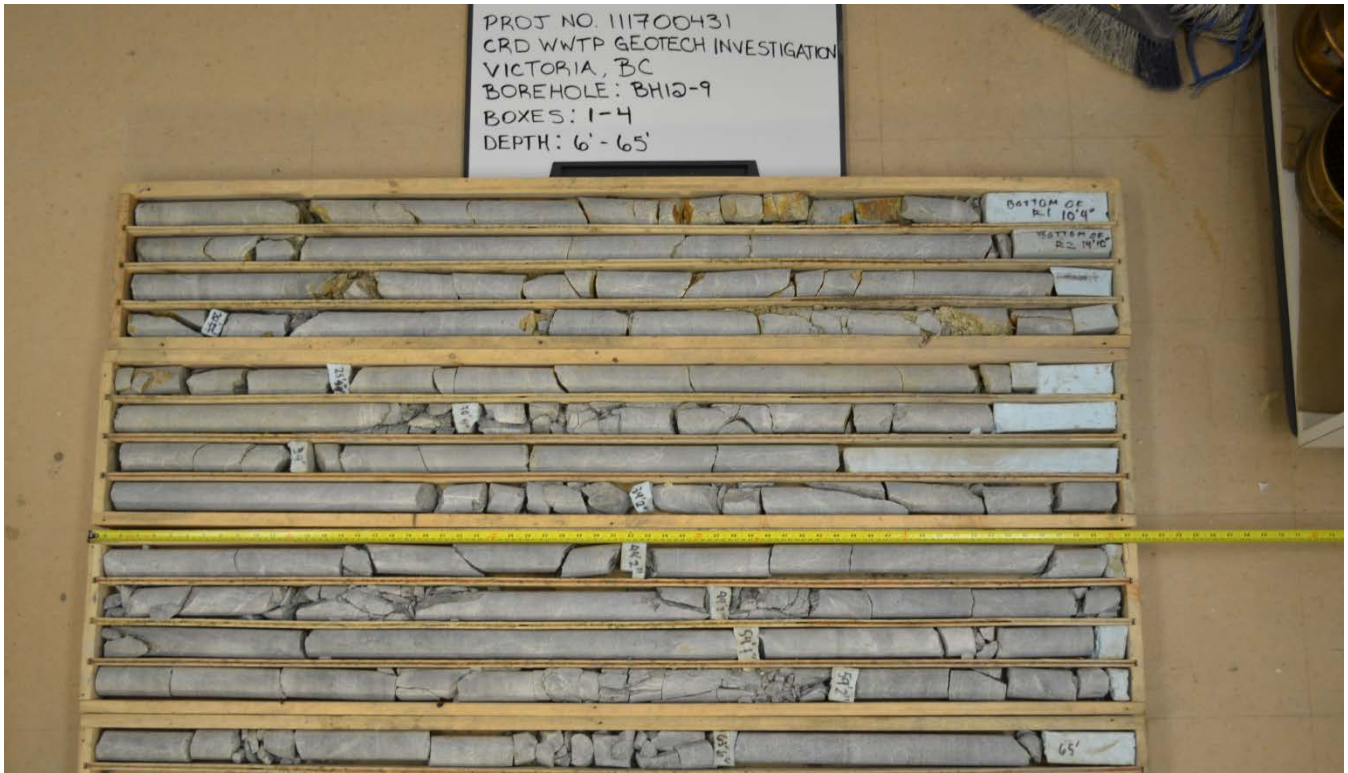
BH12-9 - Depth from 6' to 65' – Dry
