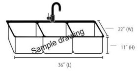
Measurements:  $36 \times 22 \times 11 = 8,172$  cubic inches Divide results by 231\* = 37.7 US gallons Multiply results by 75% = 28.275 US gallons Assign 1 minute drain down = 28.275 gpm \*Note: 231 cubic inches = 1 US gallon
