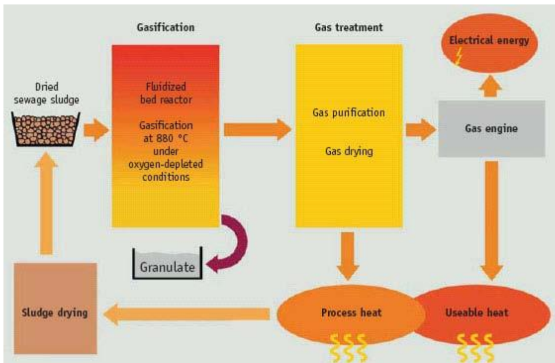
Figure 3.20 – KOPF Fluidized Bed Gasification System
