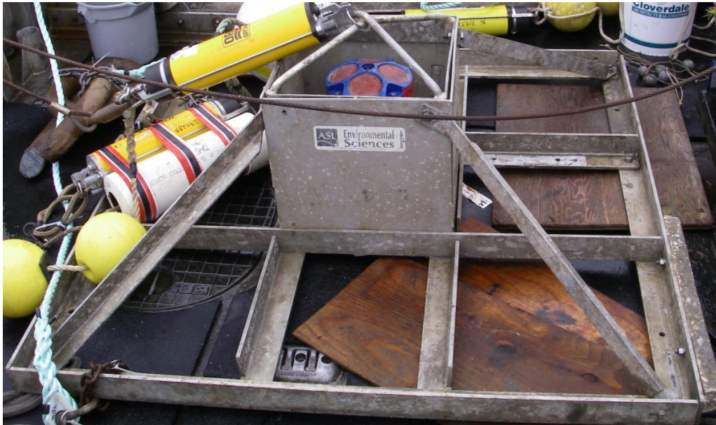
Figure 2-2. Bottom frame used for the ADCP current velocity measurements at the two Finnerty Cove sites.
