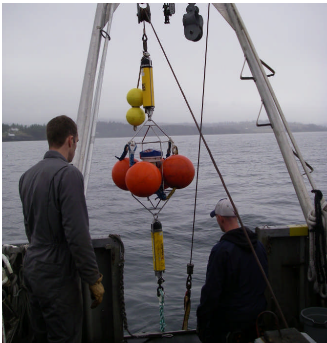
Figure 2-1. Deployment of one of the taut-line ADCP moorings off Albert Head.
