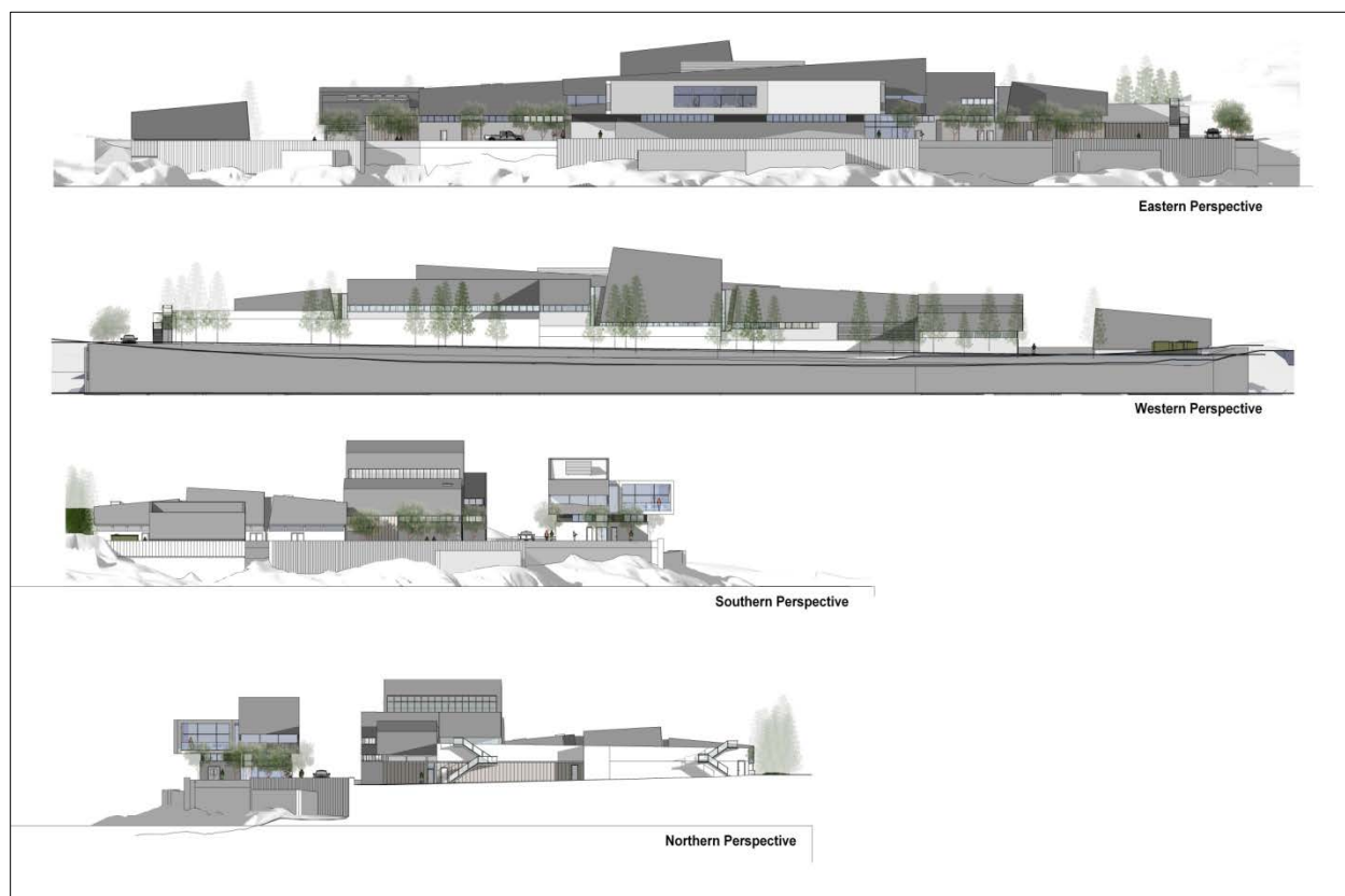
Figure 79 Massing Diagram of the Proposed McLoughlin Point Wastewater Treatment Facility Showing Structure Elevations from Different Perspectives
