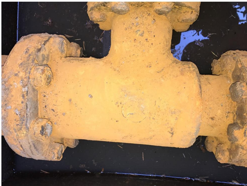
Photograph #9 – Top View: 150 mm Tee Fitting Tee Body, flanges, Nuts & Bolts
