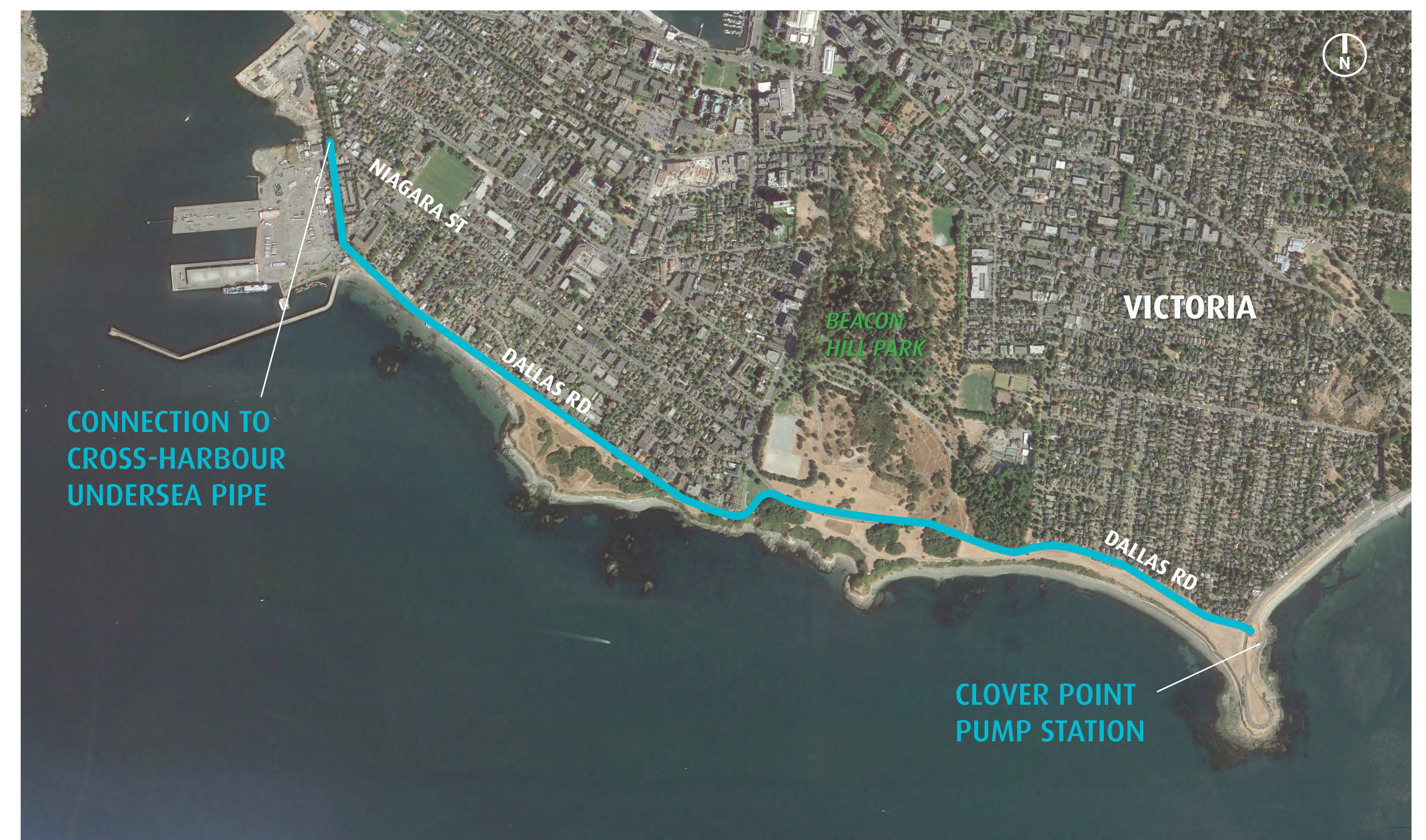
Alignment of the Clover Forcemain along Dallas Road
