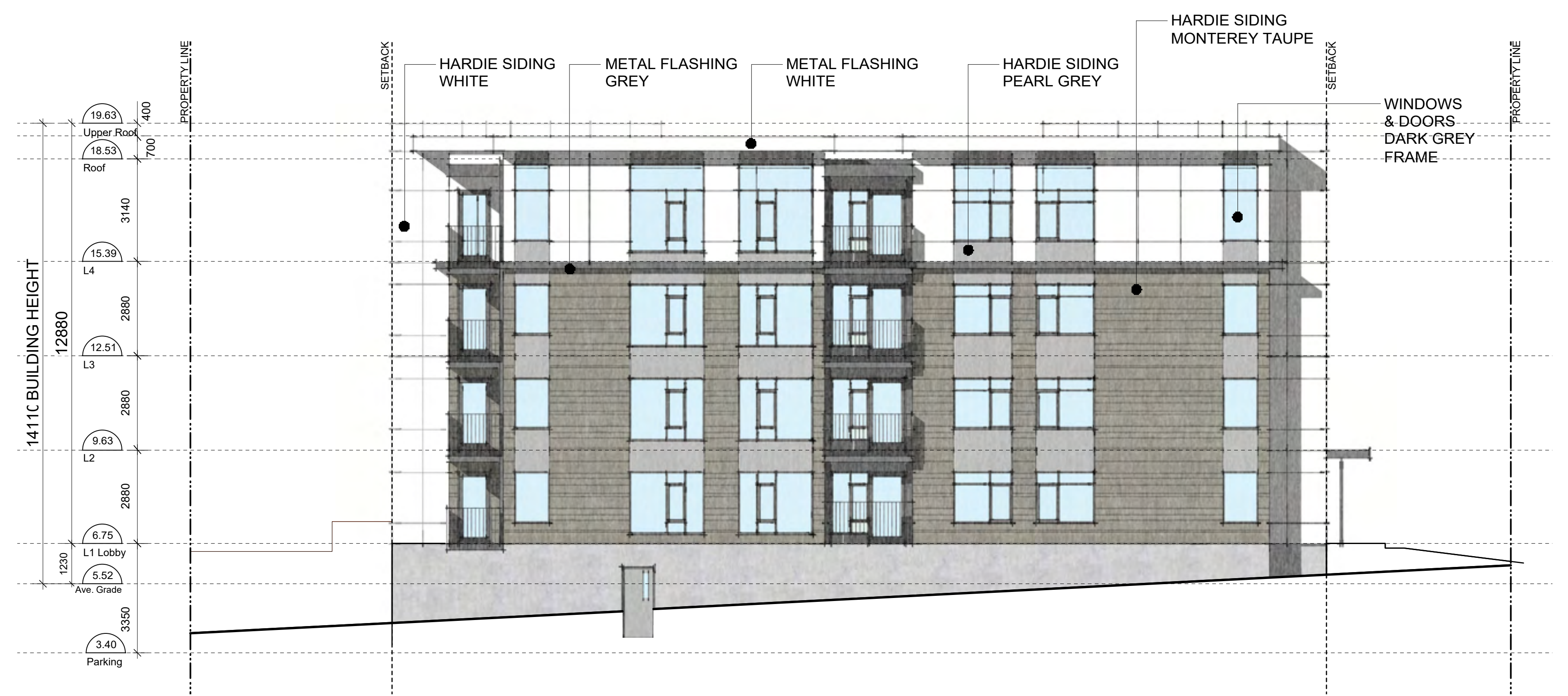
2 West Elevation / West Building Scale: 1:100 A402
