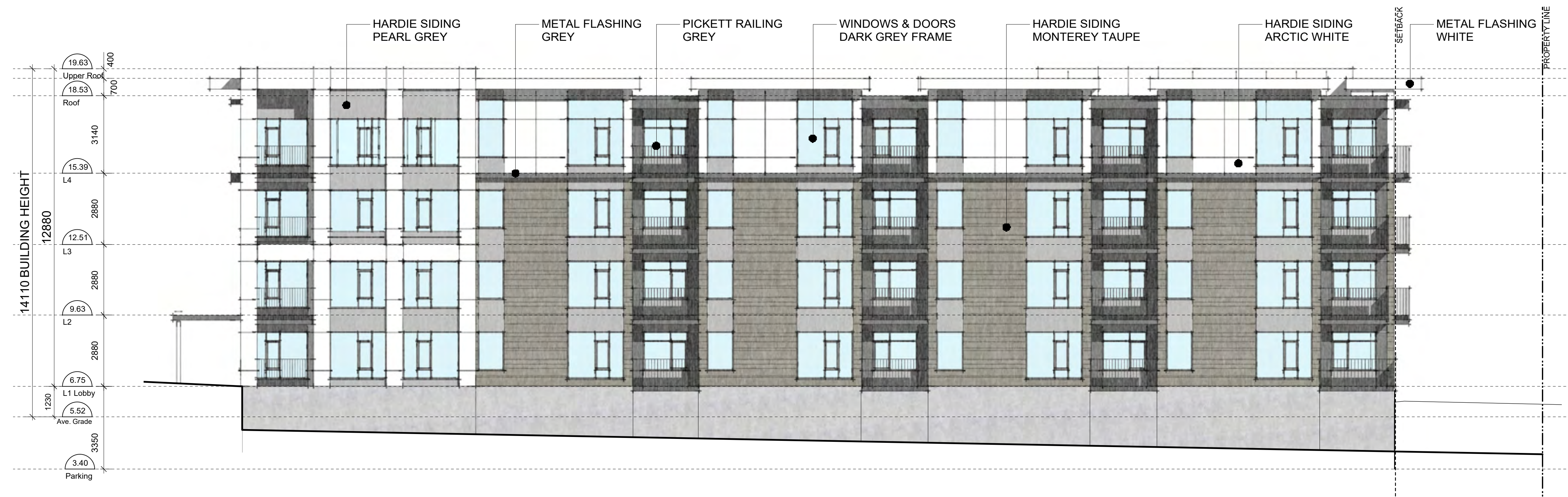
1 North Elevation / West Building Scale: 1:100 A402
