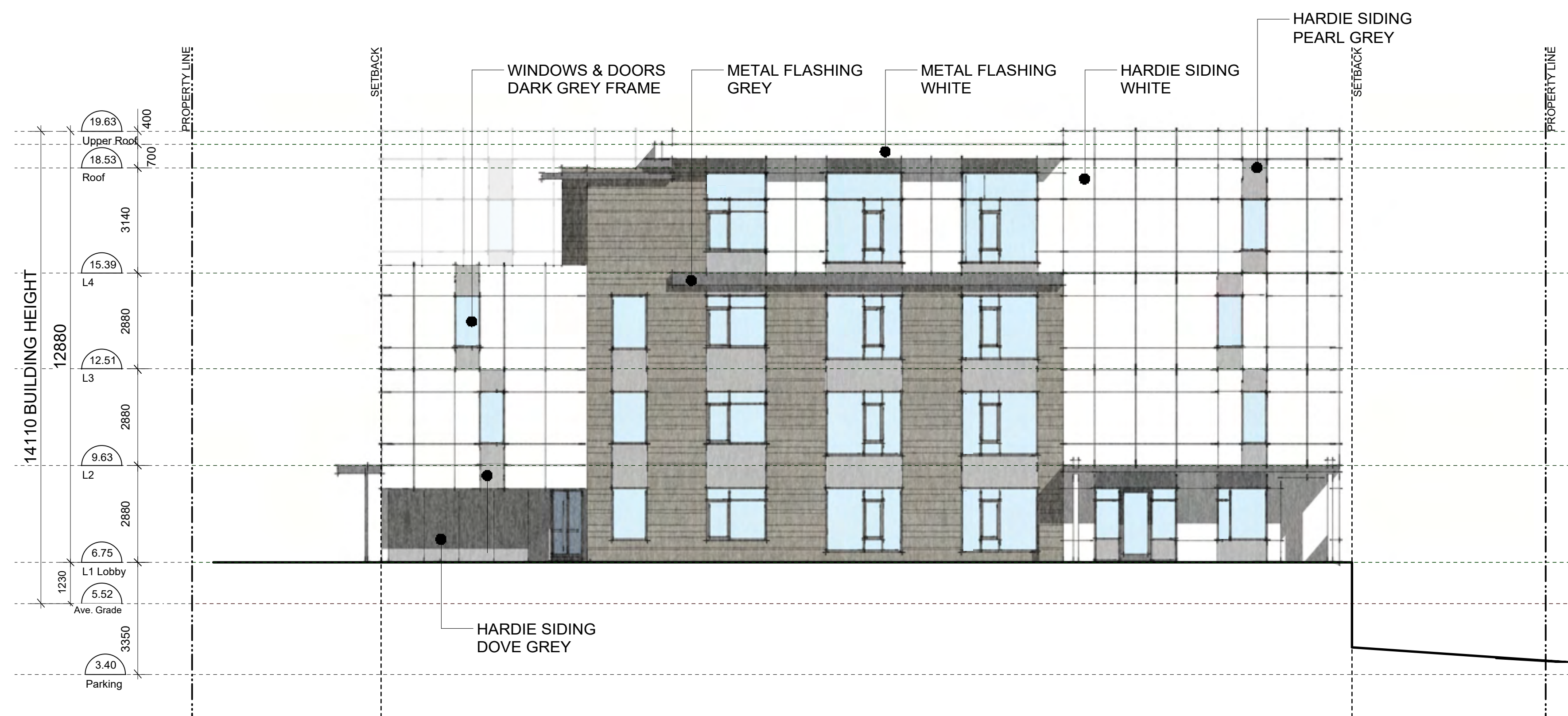
2 East Elevation / West Building Scale: 1:100
